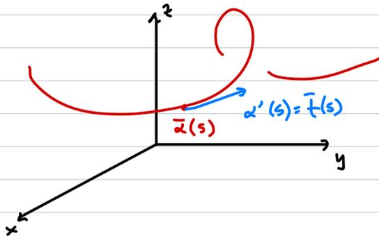
The unit tangent to  $\bar{\alpha}$  at  $s$ ,  $\bar{t}(s)$ , given by:  $\bar{\alpha}'(s)$ .
